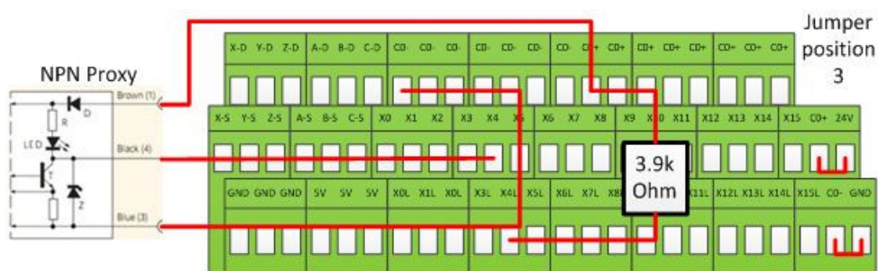
Figure 33 NPN Proxy with Internal Pullup
