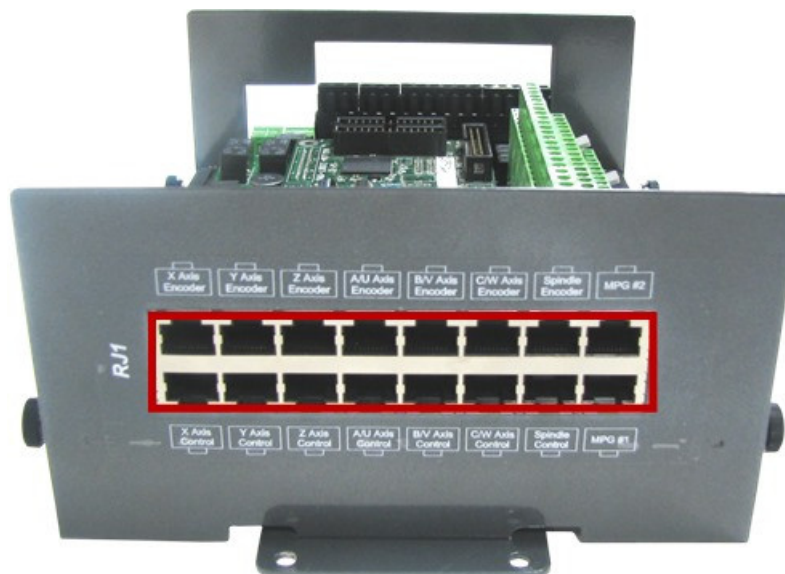
Figure 9 Differential Step and Direction, and Encoder Feedback RJ45 Connections
